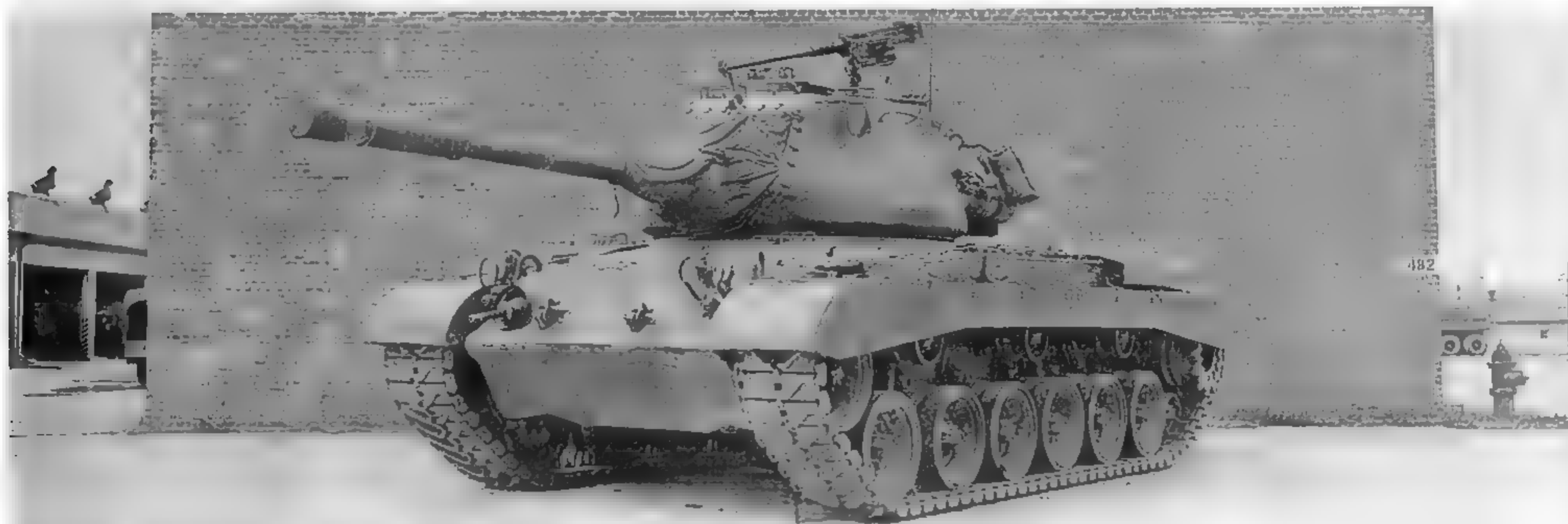
As the last U.S. tank with a co-driver, the M47 was also the last to have a ball-mount machine gun in the hull. (Photo courtesy of Patton Museum)
